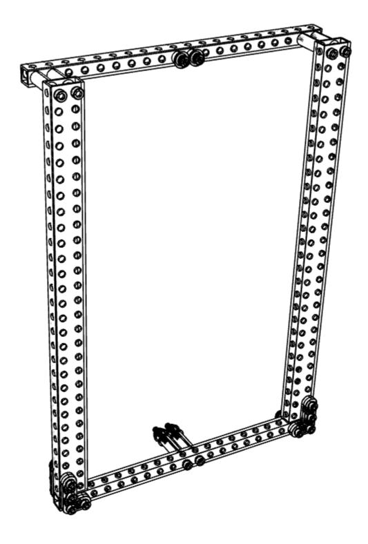
Install a total of four 2 x 3 L gussets (am-5004 $\_$ 2x3) to a 0.5 x 0.5 x 10.0 tube (am-5001-1000) using four 10-32 x 1250 screws (am-1041) and four 10-32 Nylock nuts (am-1063).
